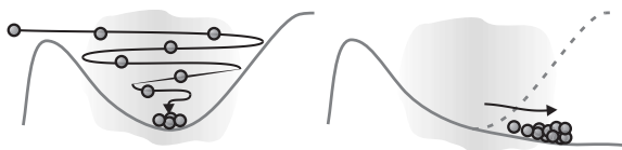
Fig. 4. Illustration of accumulation, cooling, and bunching in a buffer gas-filled ion trap.
